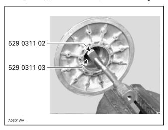
Mount puller screw head in a vise.
