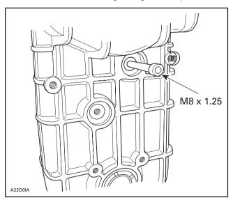
Remove intermediate gears.
