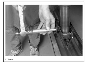
Unfasten rod nut then pull out shock from bottom. Check shock as described below in inspection. At installation, make sure bushings are in place.
