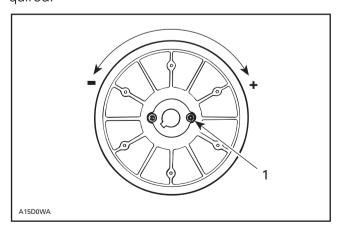
1. Allen screw with jam nut
