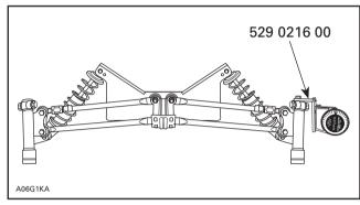
TYPICAL — DSA CAMBER ADJUSTMENT SET-UP
