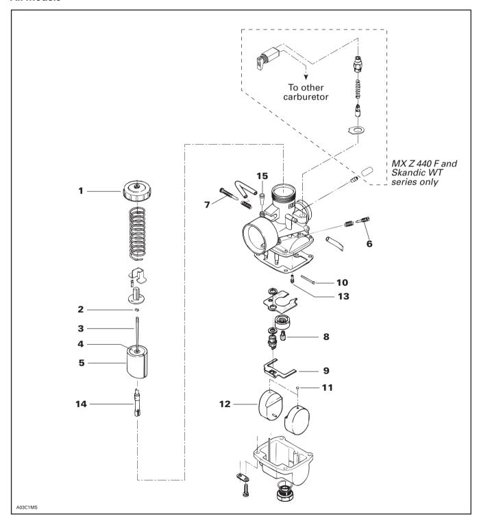
Sub-Section 11 (CARBURETOR AND FUEL PUMP)
