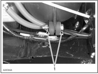
1. Remove bolt and lock nut
