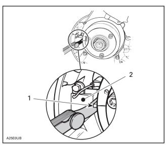
ADJUSTING TRIGGER COIL AIR-GAP
