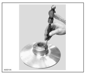
Install support plate (P/N 529 0311 03) inside sliding half.
