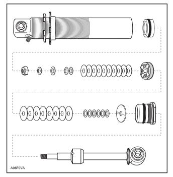
NOTE: As a general rule we suggest replacing the damper rod lock-nut after 4 rebuilds to ensure good locking friction.
