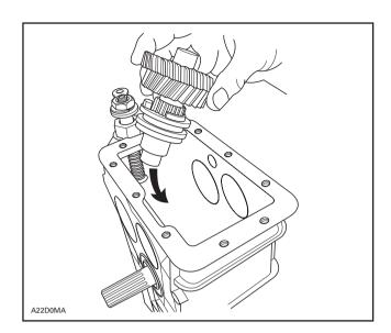
Install shim and bearing on LH side.
