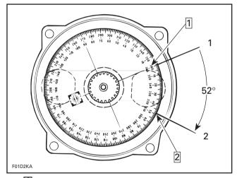
Step 1: Align 360° line of degree wheel here
