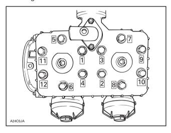
Torque screws no. 1 to 10 Nom (90 lbfoin).
