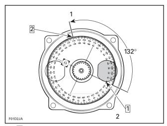
Step 1: Align 360° line of degree wheel here Step 2: Find 132° on degree wheel and mark here
