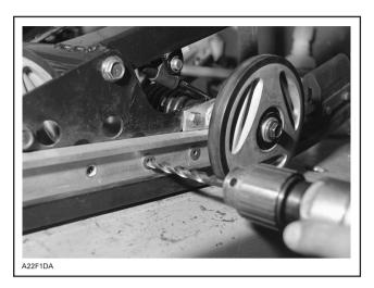
Rivets can be substitued by M8 x 20 bolts and nuts.
