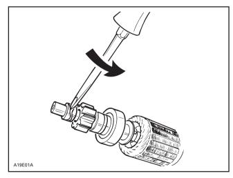
Twist screwdriver to separate stop collars no. 12 thus giving access to circlip no. 13.
