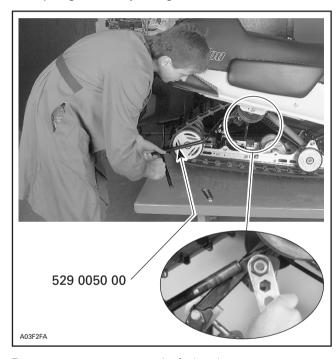
Remove nut on top end of shock.
