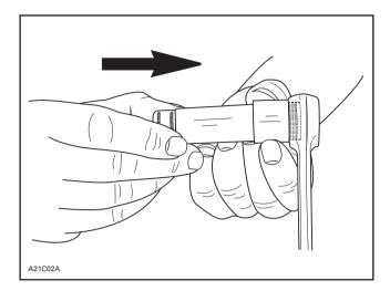
Mount piston over connecting rod with the letters "AUS" (over an arrow on the piston dome) facing in the direction of exhaust port.
