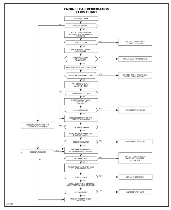
Sub-Section 04 (LEAK TEST AND ENGINE DIMENSION MEASUREMENT)
