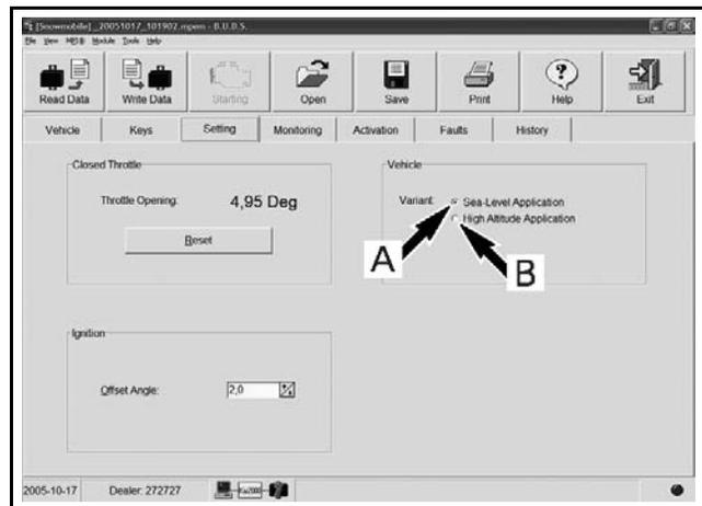
Enter B.U.D.S., select “Settings” and, when illustrated screen is showed, — select A) *Sea-Level Application* or — select B) *High Altitude Application* in the *Vehicle/Variant* box and then, click on the **Write Data** icon.
