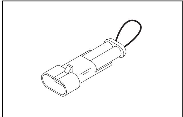
Illustration shows reverse connector (P/N 515 174 700), used at 2400 m (8000 ft) in some FAN models. — *Simply unplug existing sea level cap from the ECM and plug-in the reverse connector.*
