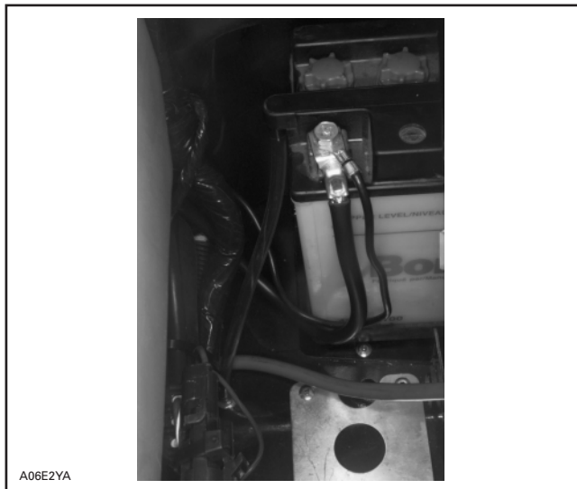
BLACK NEGATIVE (-) BATTERY CABLES POSITIONING
