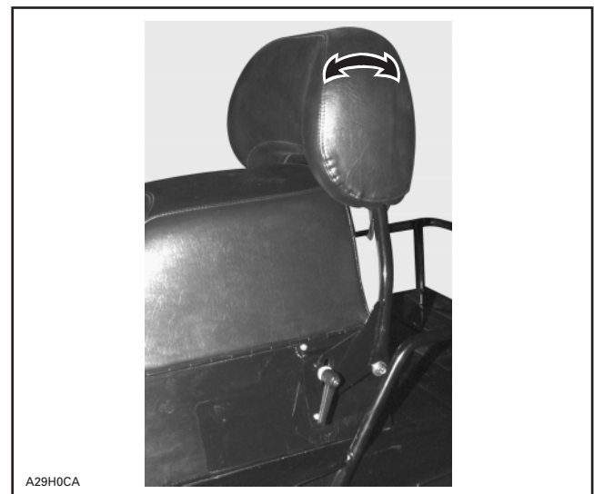
TYPICAL — BACKREST PROPERLY INSTALLED
