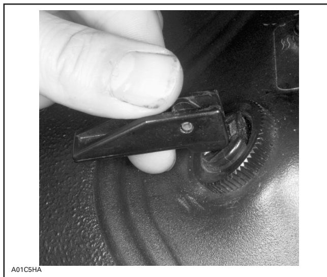
CHOKE LEVER—FULLY OPENED POSITION
