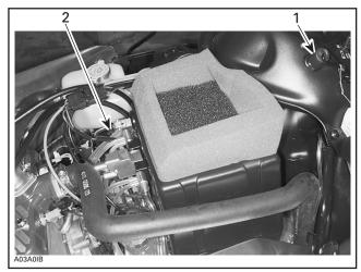
Safety lanyard switch and cap 2. MPEM
