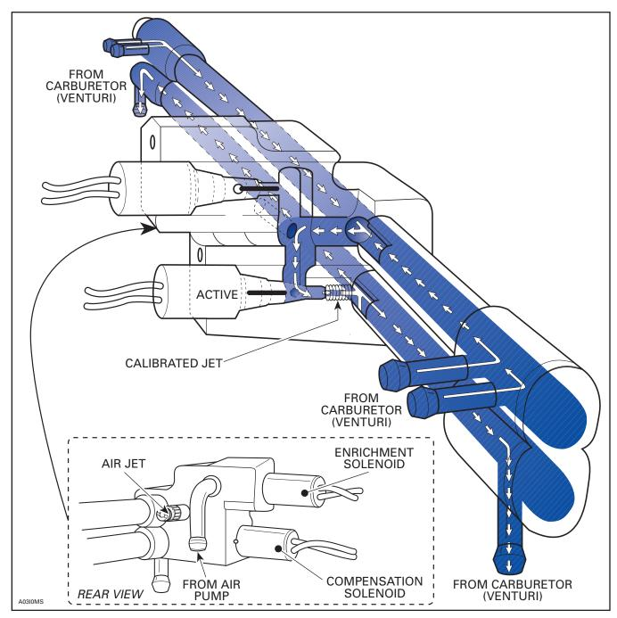
The compensation ratio will depend on the air temperature and the atmospheric pressure.
