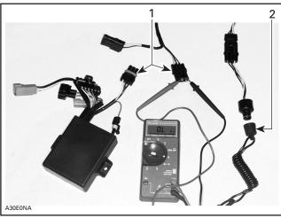
TYPICAL — HARNESS REMOVED FOR CLARITY Housing disconnected 1. 2. DESS cap remove
