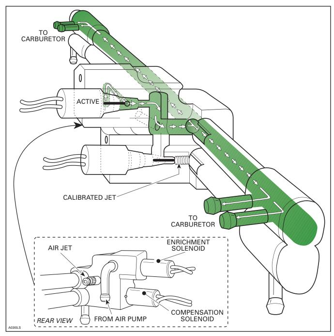
This enrichment mode of the air/fuel mixture takes place at start-up and during engine warm-up, and it depends on engine temperature.
