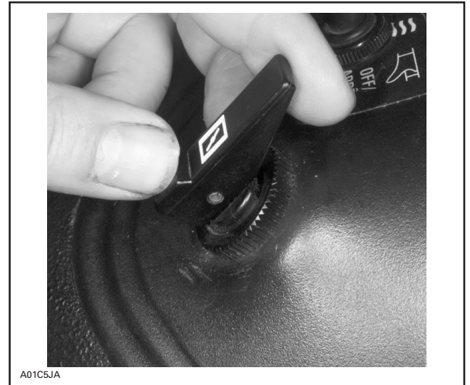
CHOKE LEVER — CLOSED POSITION
