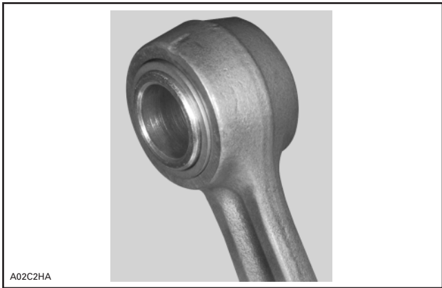
TYPICAL — CAGELESS BEARING AND SLEEVE INSTALLED
