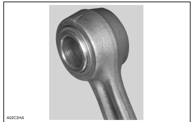
TYPICAL — CAGELESS BEARING AND SLEEVE INSTALLED
