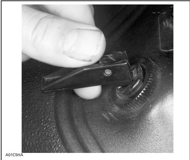
CHOKE LEVER — FULLY OPEN POSITION
