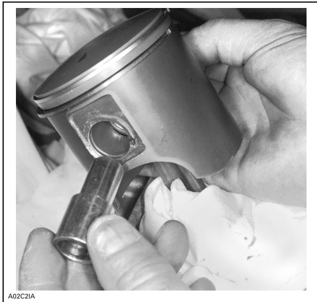
TYPICAL — SHOULDERED SLEEVE INSTALLATION
