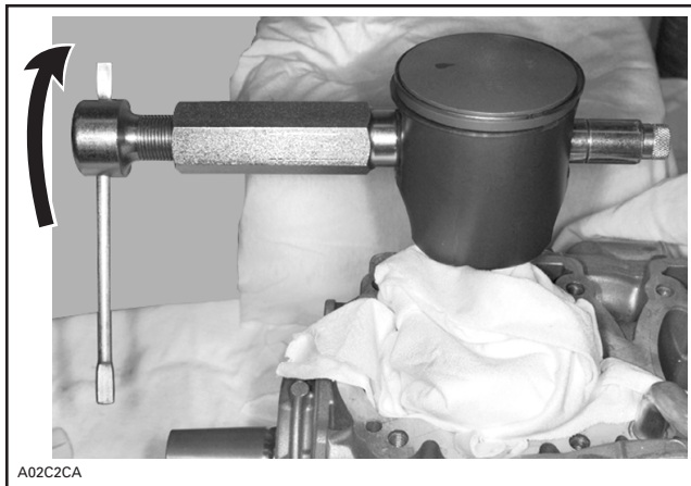
TYPICAL — PISTON PIN EXTRACTION
