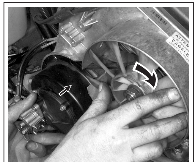
TURN FAN TO SLIDE OIL PUMP SHAFT IN PLACE
