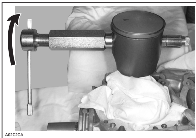
TYPICAL — PISTON PIN EXTRACTION
