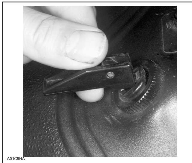
CHOKE LEVER — FULLY OPEN POSITION
