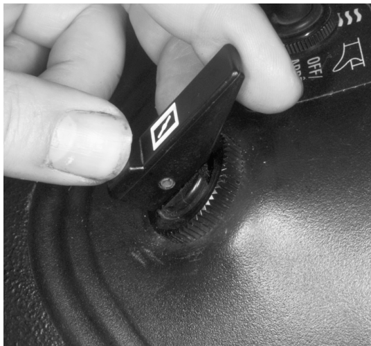
CHOKE LEVER — CLOSED POSITION
