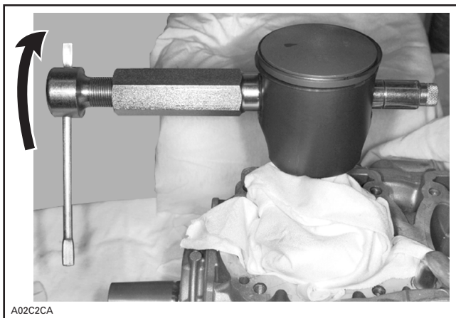
TYPICAL — PISTON PIN EXTRACTION
