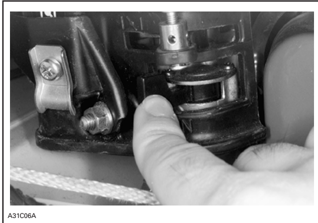
FUEL VALVE TO "OFF" POSITION
