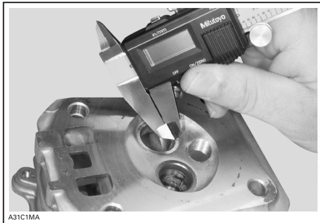
VALVE SEAT WIDTH
