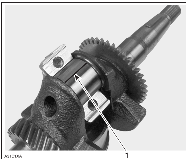
1. Plastigauge properly positioned
