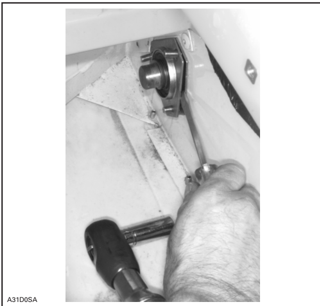
DETACH BEARING HOLDER HALVES
