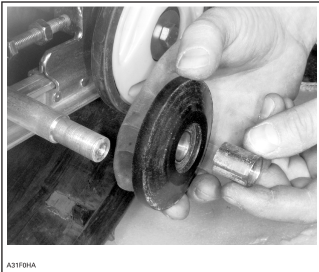
CHECK BUSHING, WHEEL AND SHAFT CONDITION
