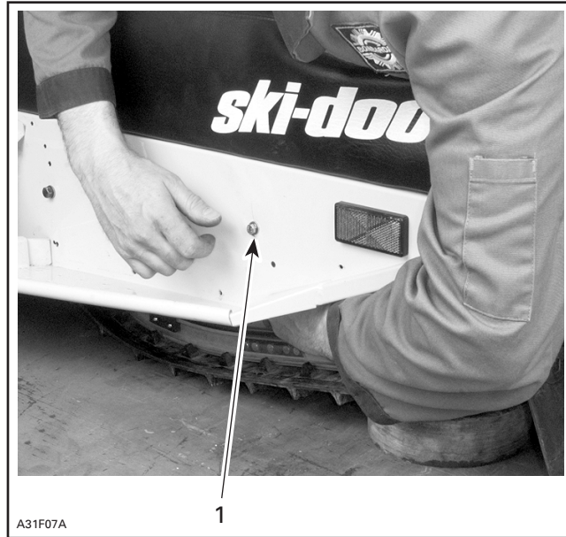
A31F07A 1. Unscrew upper idler wheel axle
