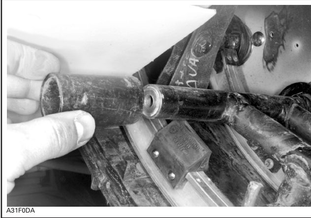
REMOVE AND CLEAN BUSHING
