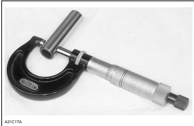
MEASURE PISTON PIN
