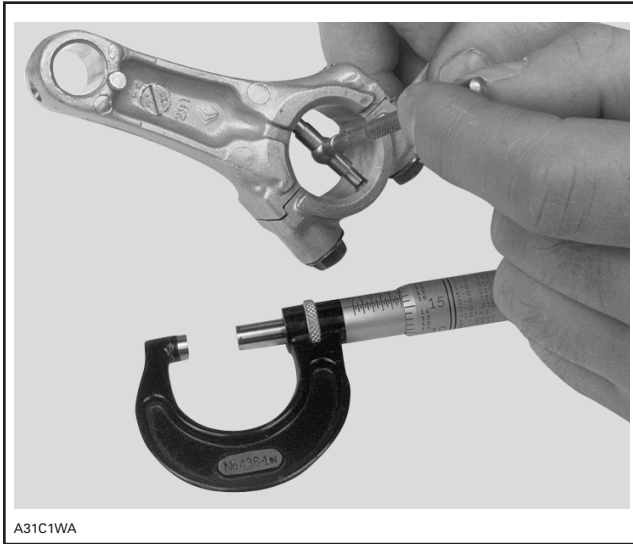
MEASURE CONNECTING ROD BIG END
