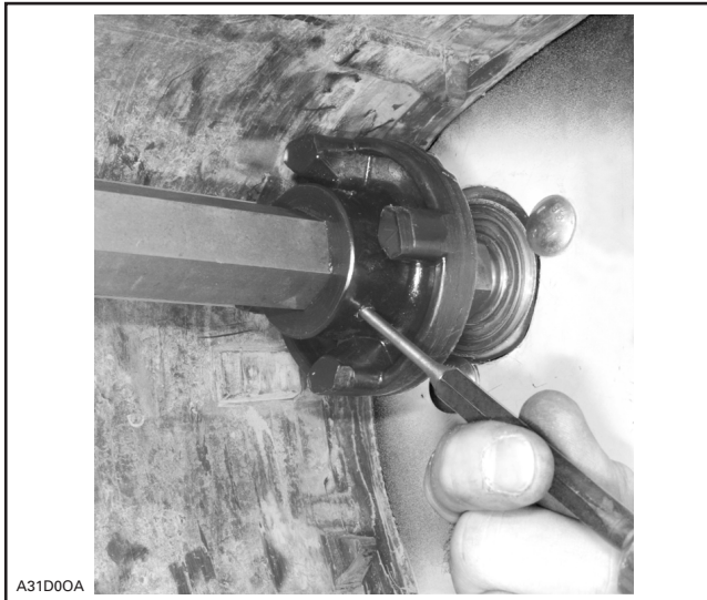
REMOVE SPRING PIN
