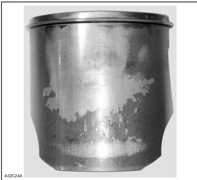
PISTON WITH MOLYKOTE COATING WORN OFF
