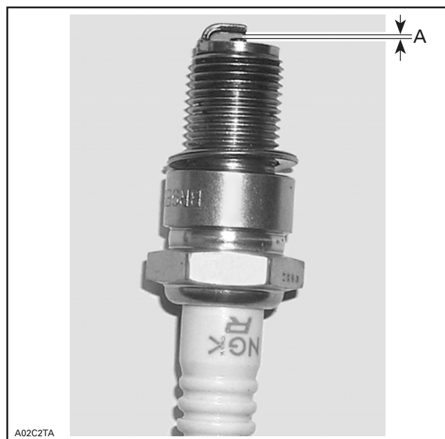
A. Gap specification is 0.45 mm \pm 0.05 mm (0.018 \pm 0.002 in)
