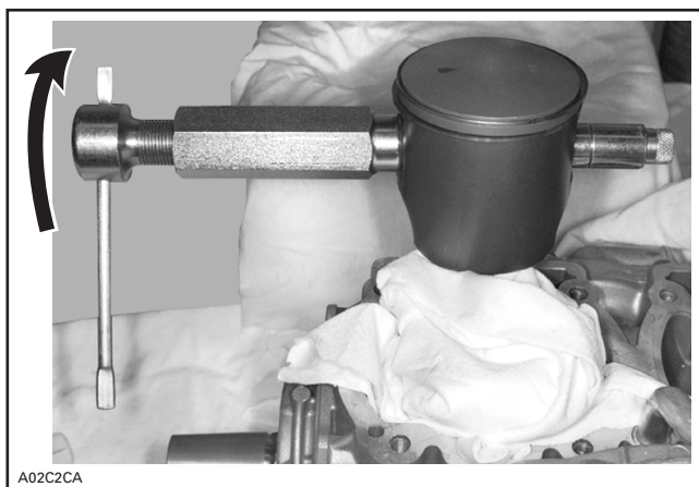
TYPICAL — PISTON PIN EXTRACTION
