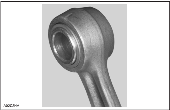
TYPICAL — CAGELESS BEARING AND SLEEVE INSTALLED Mount piston over connecting rod with the letters “AUS” (over an arrow on the piston dome) facing in the direction of exhaust port.
