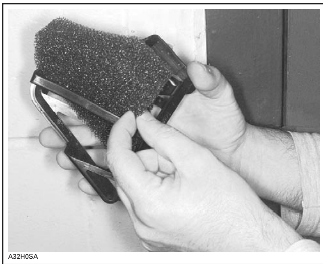
REMOVAL OF FILTER FROM ITS GRILL
