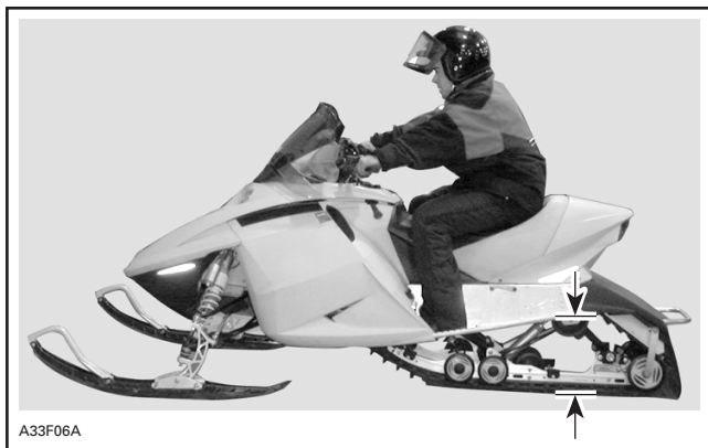
TYPICAL — TOO HARD OF ADJUSTMENT
