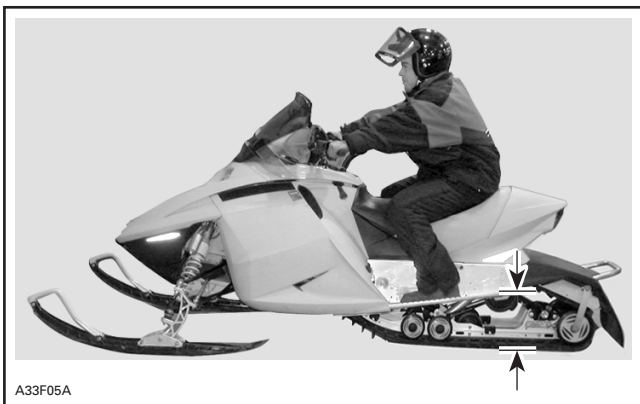
TYPICAL — TOO SOFT OF ADJUSTMENT
