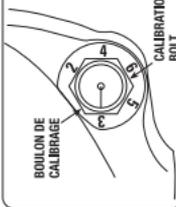
Adjust all three drive pulley bolts to same position.
