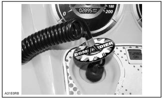
TETHER CORD CAP INSTALLED ON POST
