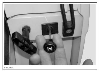
CHOKE IS ENGAGED FOR COLD ENGINE STARTING
