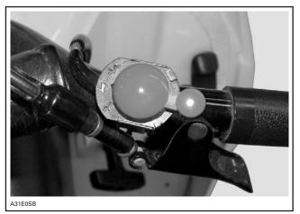
ENGINE CUT-OUT SWITCH TO MIDDLE POSITION
