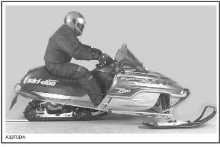
TYPICAL — TOO HARD OF ADJUSTMENT (REAR SUSPENSION RUNS TOO HIGH, IT HAS COLLAPSED LESS THAN 50 mm (2 in)
