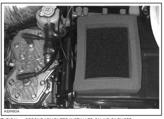
TYPICAL — SECONDARY FILTER INSTALLED ON AIR SILENCER
