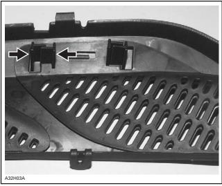
TO CLOSE, SQUEEZE CLOSING TABS BETWEEN THUMB AND INDEX
