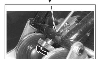
1. Loosen lock nut, turn knob accordingly then retighten lock nut
