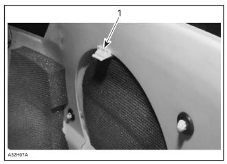
1. Push tab down and remove panel out of bottom pan
