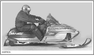
TYPICAL — TOO SOFT OF ADJUSTMENT (REAR SUSPENSION IS TOO LOW, IT HAS COLLAPSED MORE THAN 75 mm (3 in)
