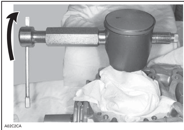
TYPICAL — PISTON PIN EXTRACTION
