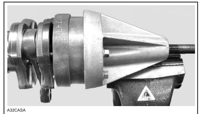
BEARING PULLER SECURED IN THE VISE
