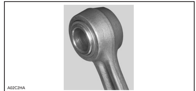
TYPICAL — CAGELESS BEARING AND SLEEVE INSTALLED
