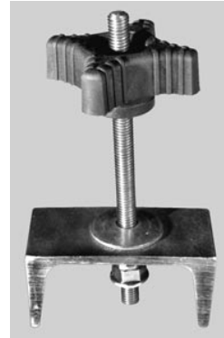
Driven pulley spring compressor (P/N 529 035 300)
