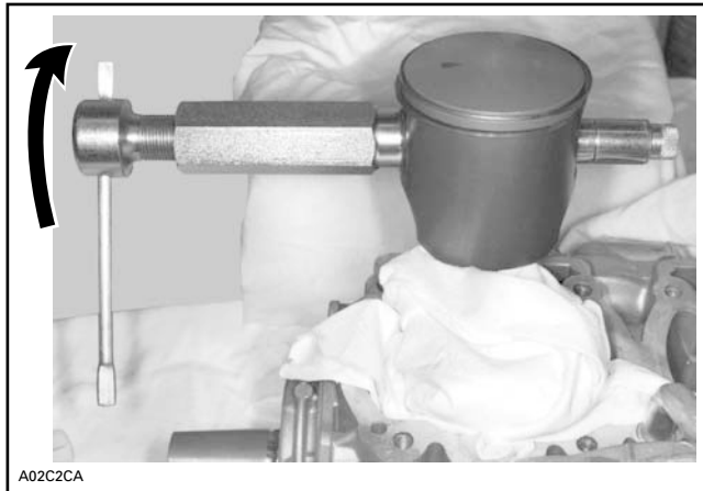
TYPICAL — PISTON PIN EXTRACTION
