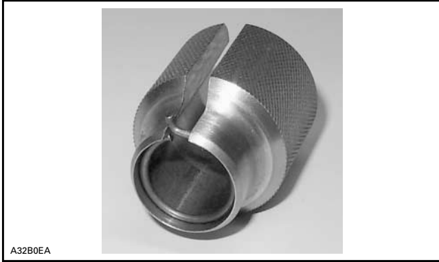
CIRCLIP READY TO BE INSTALLED ON PISTON
