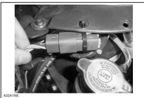
**NOTE:** The use of the power supply harness [1] will keep the vehicle's ECM ON. Not using it will make the ECM shut off after a few seconds.
