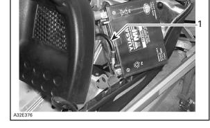
• Install the battery [1] in its support with the battery posts facing rearward.
