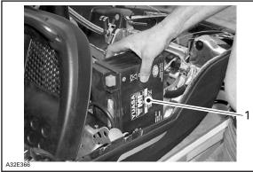
Disconnect the BLACK negative cable [1] from the battery negative post.
