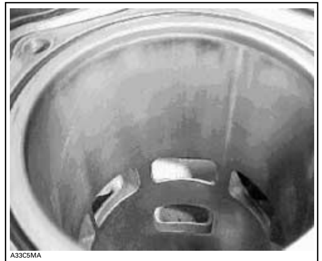
NORMAL WEAR ON A CYLINDER WALL
