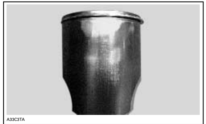
NORMAL MOLY COAT WEAR ON A PISTON
