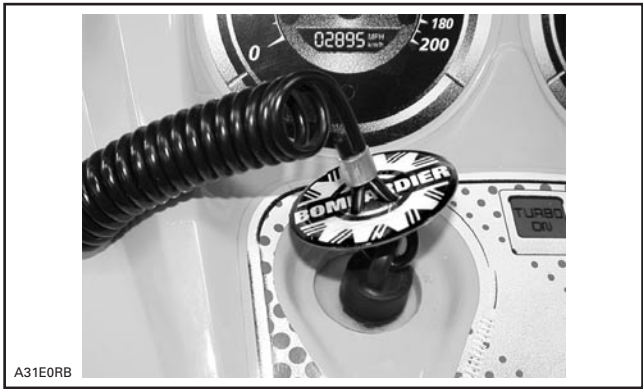
TETHER CORD CAP INSTALLED ON POST
