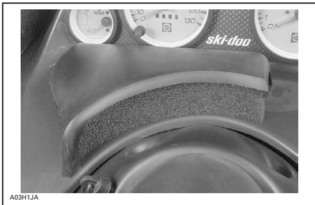
TYPICAL — FILTER INSTALLED
