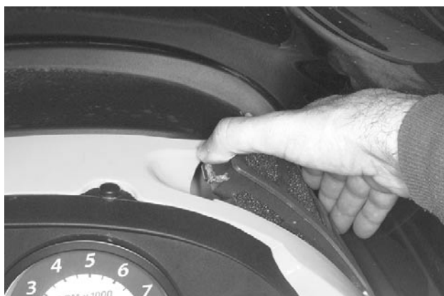
REMOVAL OF RIGHT SIDE PRIMARY FILTER GRILL
