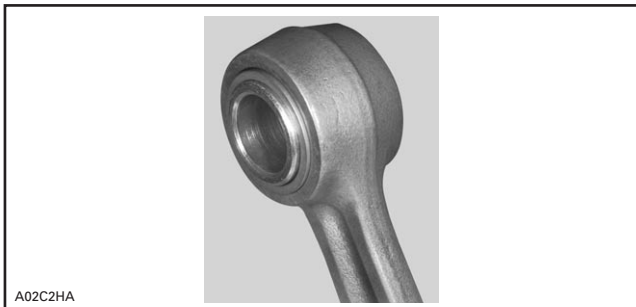
TYPICAL — CAGELESS BEARING AND SLEEVE INSTALLED
