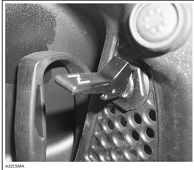
TYPICAL — CHOKE LEVER — HALF OPEN POSITION
