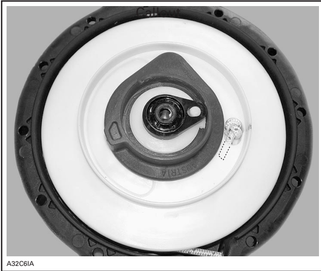
FREE PORTION INSERTED INTO SHEAVE
