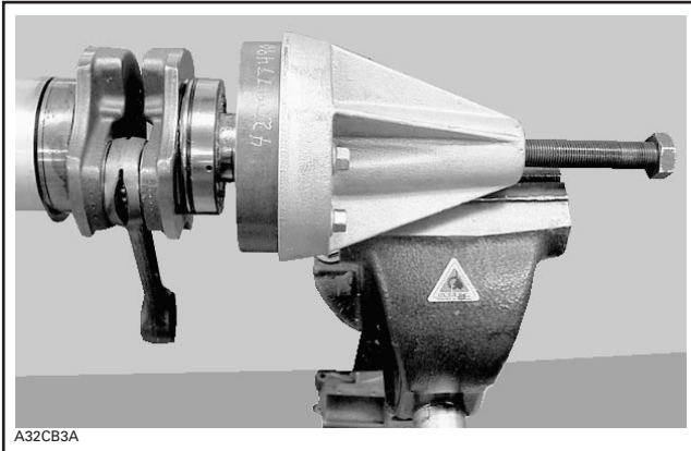
BEARING PULLER SECURED IN THE VISE
