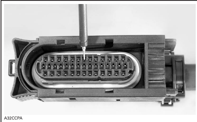
PROBE ONLY ON THE PIN NOZZLE OF FEMALE CONNECTOR
