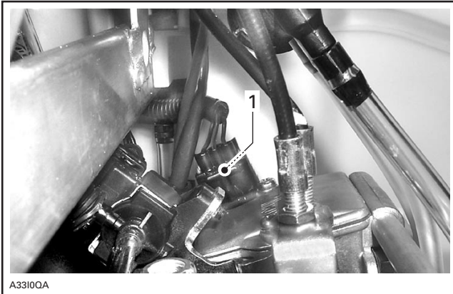
TPS CONNECTOR 1. Release button
