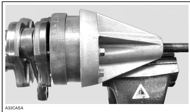
BEARING PULLER SECURED IN THE VISE
