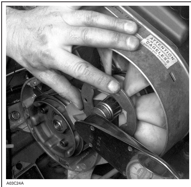
TYPICAL — TORQUE FAN NUT USING HOLDER WRENCH
