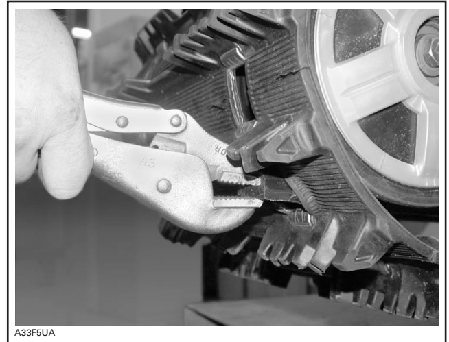
TYPICAL — PULL ON SLIDER SHOE TO REMOVE
