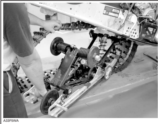
TYPICAL — REMOVE SUSPENSION
