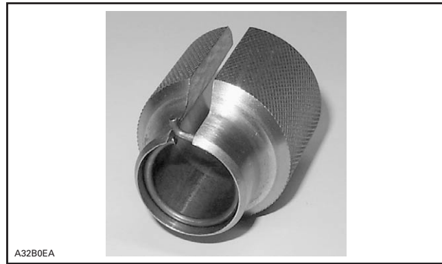
CIRCLIP READY TO BE INSTALLED ON PISTON
