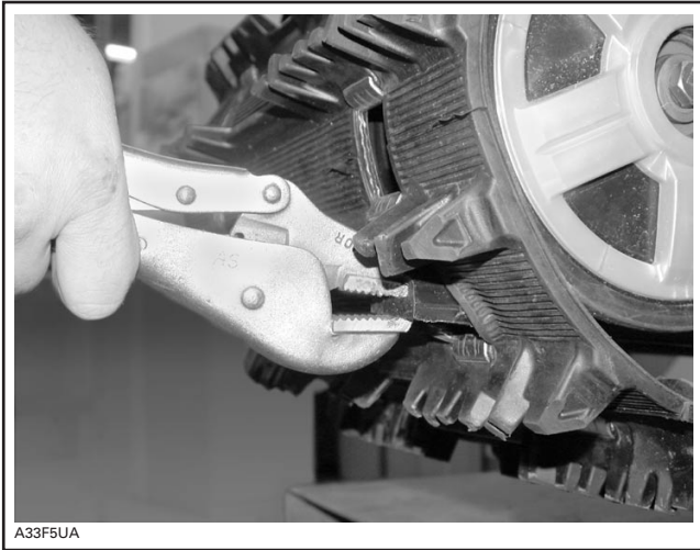
TYPICAL — PULL ON SLIDER SHOE TO REMOVE
