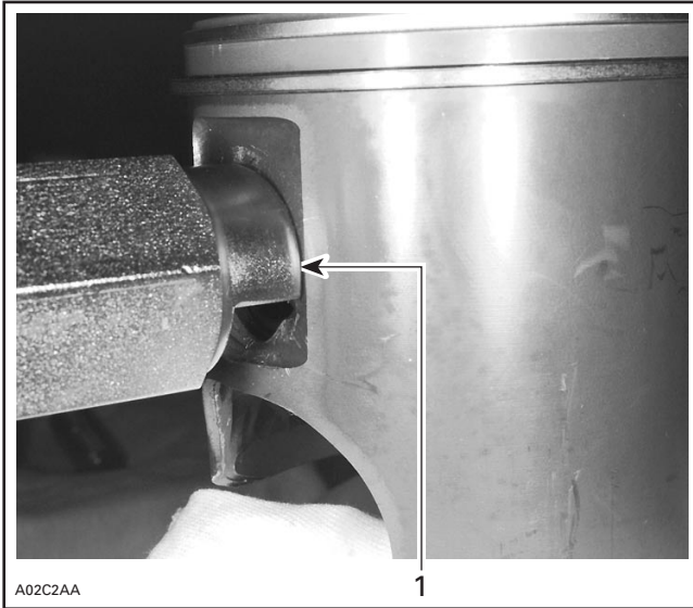
TYPICAL 1. Properly seated all around
