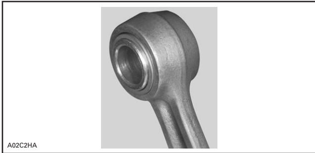
TYPICAL — CAGELESS BEARING AND SLEEVE INSTALLED
