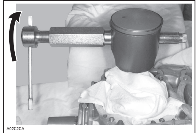
TYPICAL — PISTON PIN EXTRACTION
