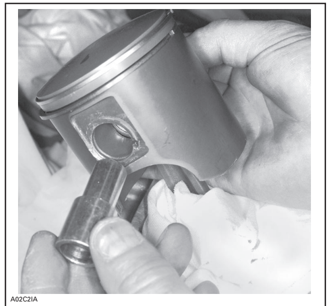
TYPICAL — SHOULDERED SLEEVE INSTALLATION
