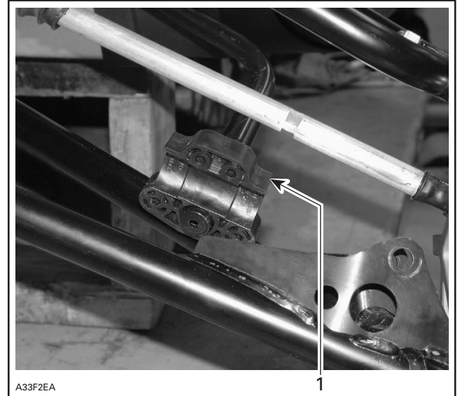
1. Temporarily rotate block by 180° for its insertion
