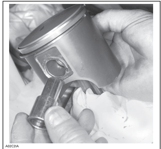
TYPICAL — SHOULDERED SLEEVE INSTALLATION
