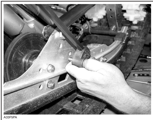
TYPICAL — REMOVE SPRING SUPPORTS
