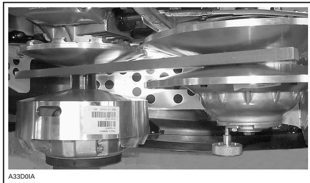
ALIGNMENT BAR IN PULLEYS
