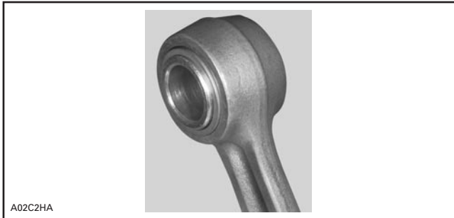
TYPICAL — CAGELESS BEARING AND SLEEVE INSTALLED
