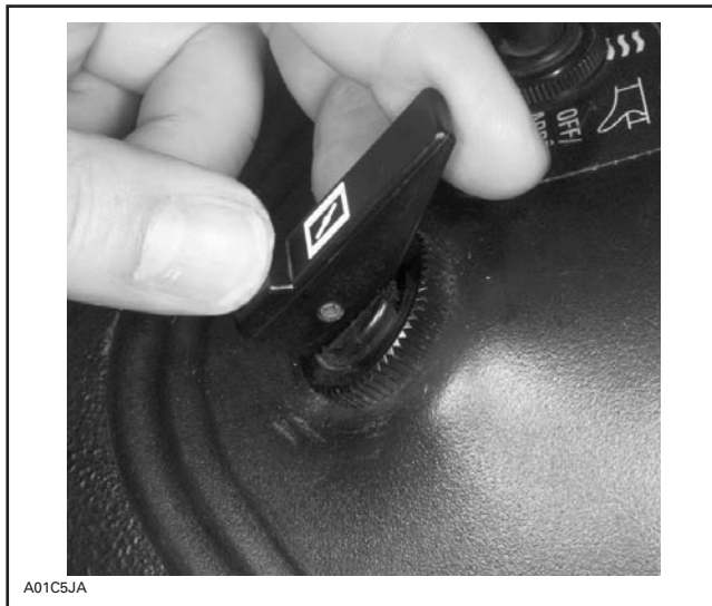
CHOKE LEVER — CLOSED POSITION
