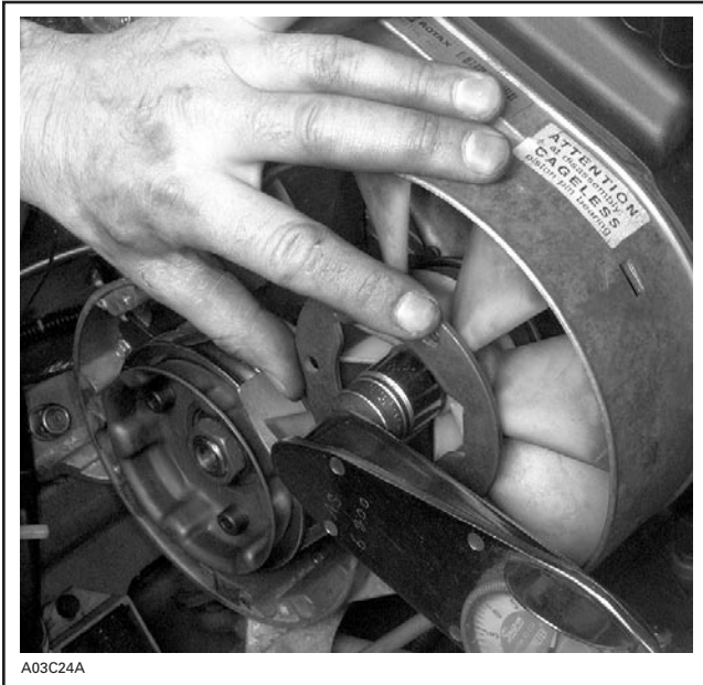
TORQUE FAN NUT USING HOLDER WRENCH
