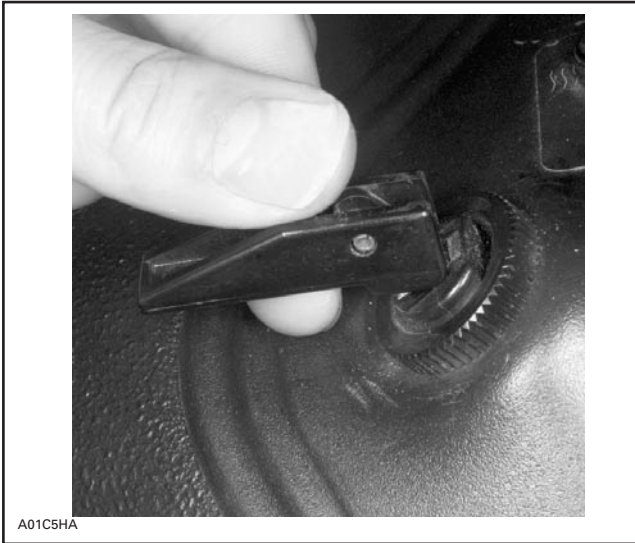
CHOKE LEVER — FULLY OPEN POSITION
