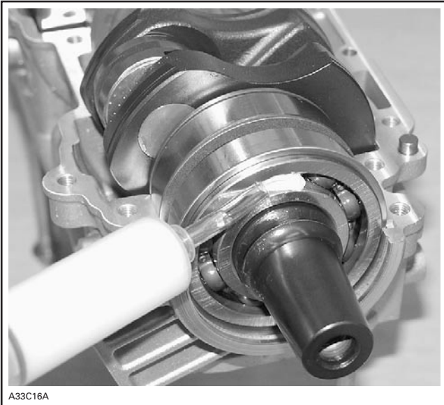
BALLS COATED WITH A SEAM OF GREASE
