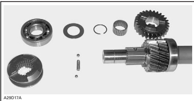
DRIVEN PULLEY SHAFT COMPONENTS
