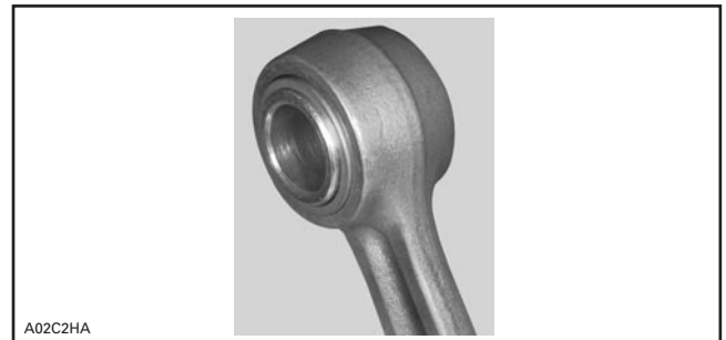
TYPICAL — CAGELESS BEARING AND SLEEVE INSTALLED
