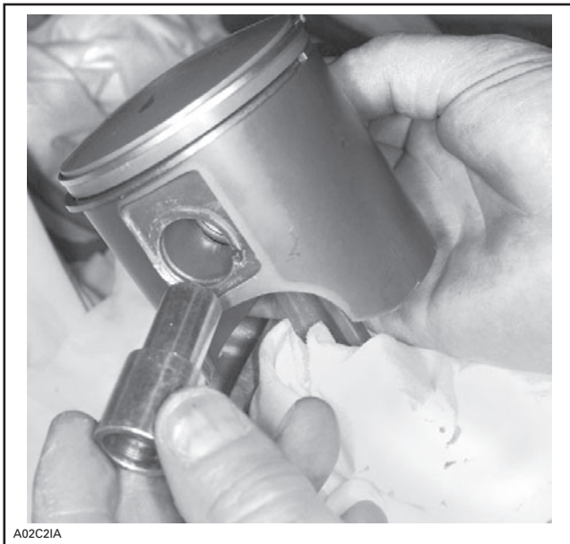
TYPICAL — SHOULDERED SLEEVE INSTALLATION
