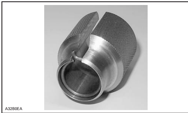
CIRCLIP READY TO BE INSTALLED ON PISTON
