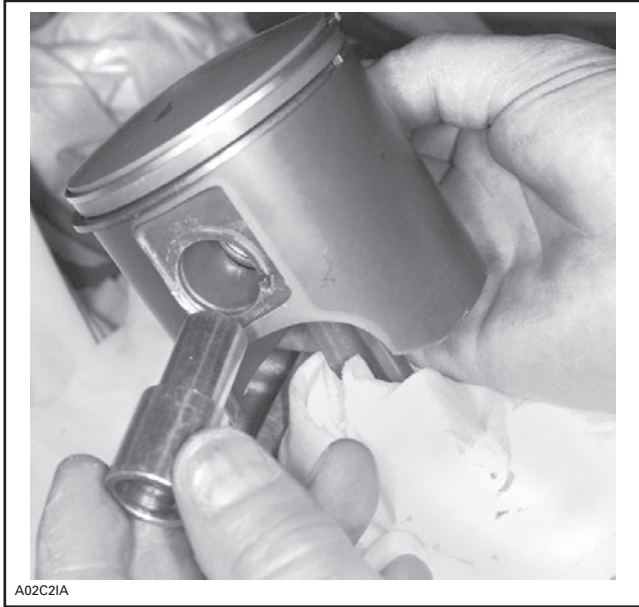
TYPICAL — SHOULDERED SLEEVE INSTALLATION
