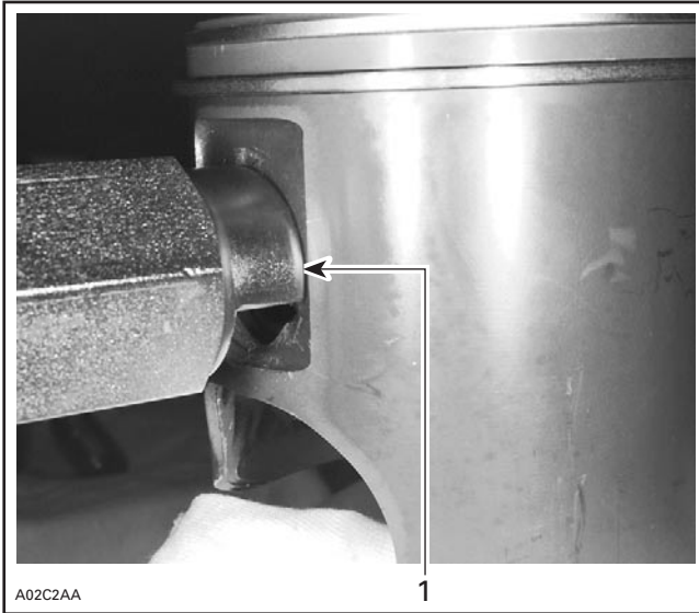
TYPICAL 1. Properly seated all around
