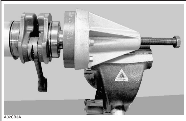
A32CB3A BEARING PULLER SECURED IN THE VISE
