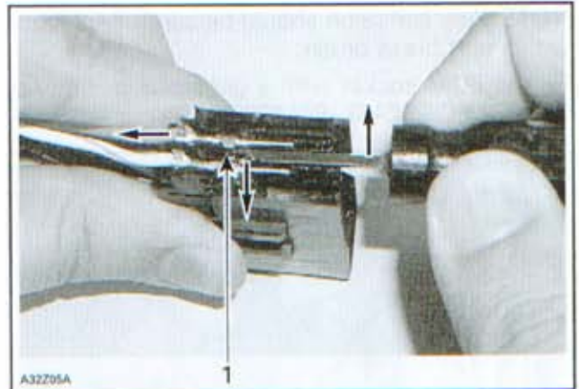
FEMALE HOUSING — CUT-AWAY 1. Lock
