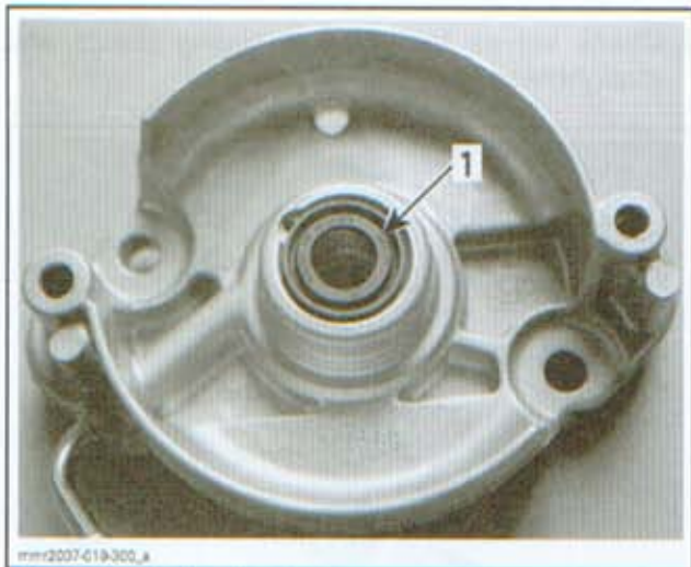
1. Lettering of oil seal on top
