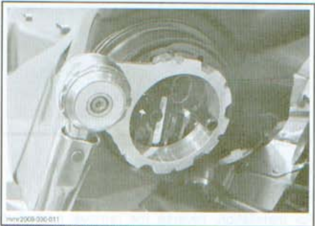
mmv2009-030-011 TORQUE WRENCH AT 90°
