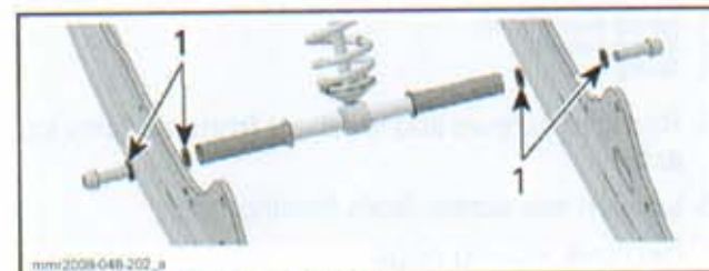
BOTTOM OF SHOCK ABSORBER 1. Washers location
