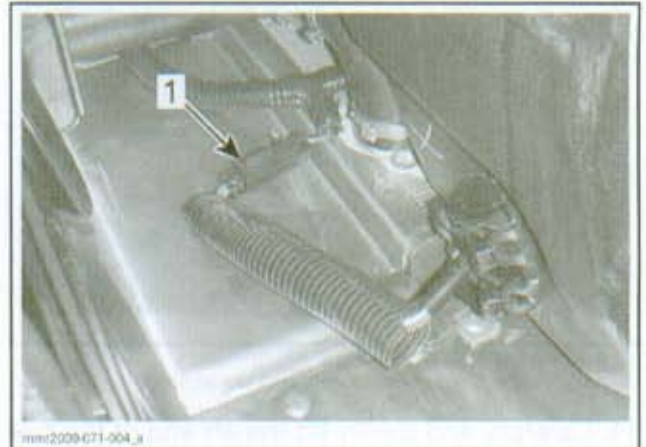
1. Fuel level sensor connector to disconnect
