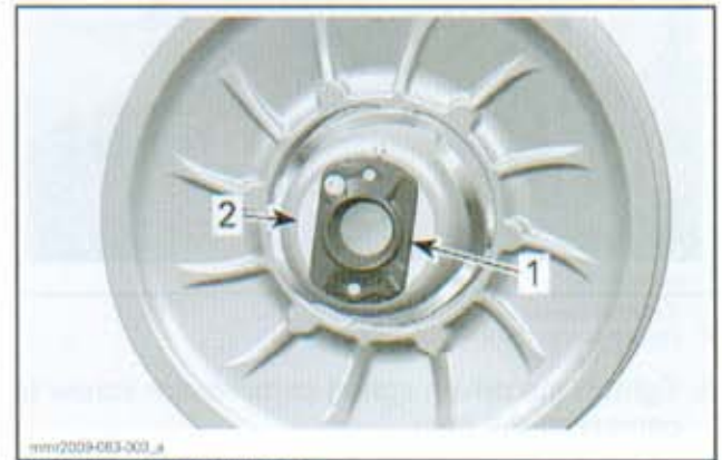
SCREW TYPE ADJUSTER 1. Adjuster hub 2. Washer
