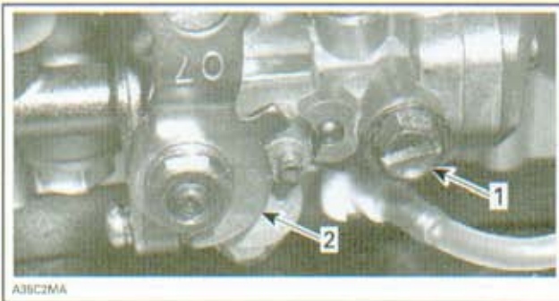
TYPICAL 1. Bleeder screw 2. Oil pump lever
