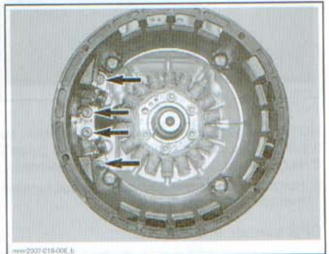
TRIGGER COIL RETAINING SCREWS
