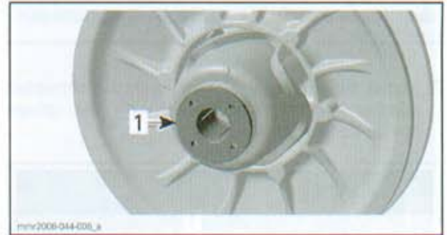
RING TYPE ADJUSTER 1. Adjusting ring
