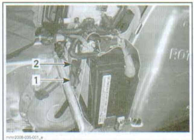
TYPICAL - 500SS/600/800R 1. START/RER fuse (FB) 2. Charging fuse (FA)
