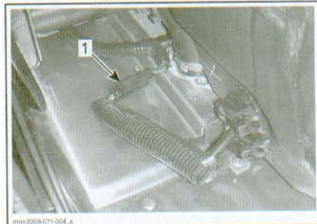
1. Fuel sensor connector to disconnect
