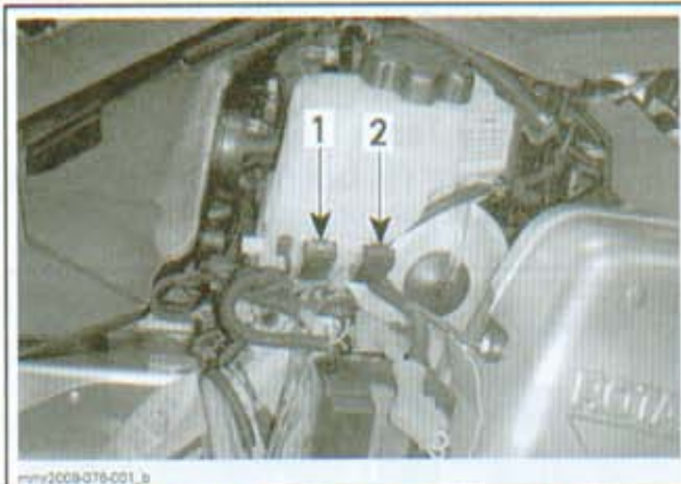
TYPICAL - FUSE LOCATIONS (ELECTRIC START MODEL)
