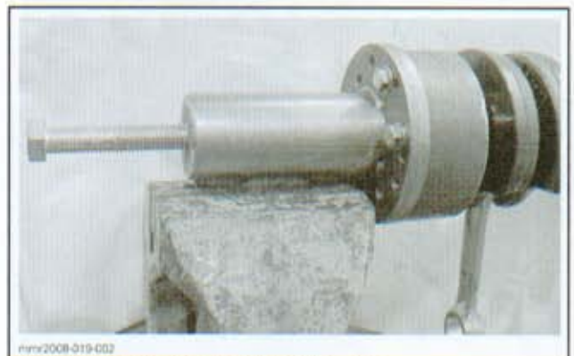
BEARING PULLER SECURED IN THE VISE
