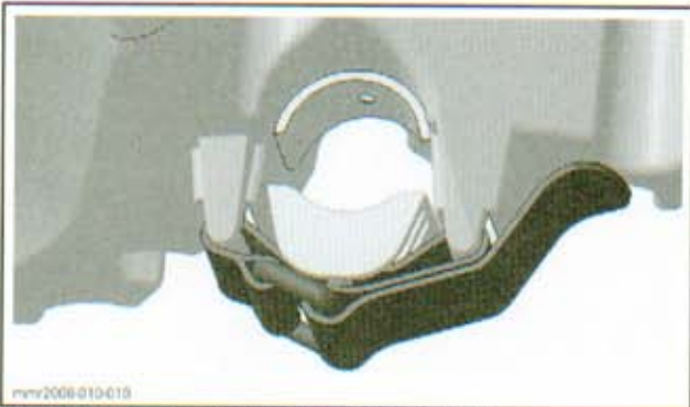
TYPICAL — REAR VELCRO STRAP ROUTING
