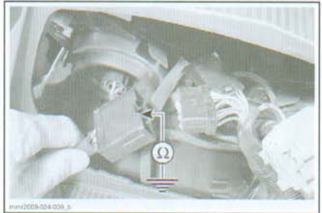
TYPICAL - STEERING HARNESS TO GROUND
