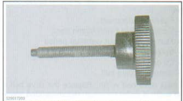
DRIVEN PULLEY OPENING TOOL (P/N 529 017 200)
