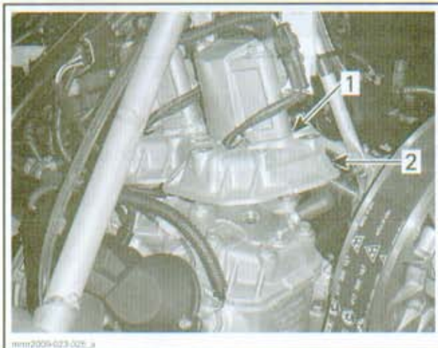
1. Thermal insulator 2. Old E-TEC cylinder head
