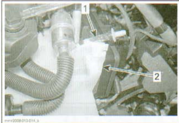
TYPICAL 1. Check valve outlet hose 2. Oil tank
