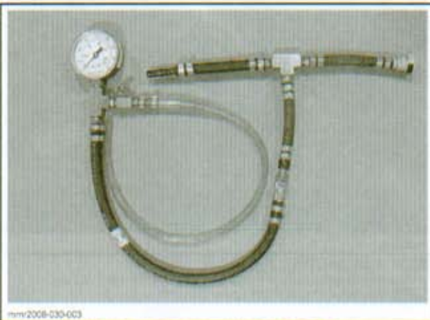
PRESSURE GAUGE WITH FUEL HOSE ADAPTER
