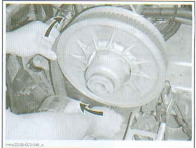
MANUALLY ROTATE DRIVE BELT
