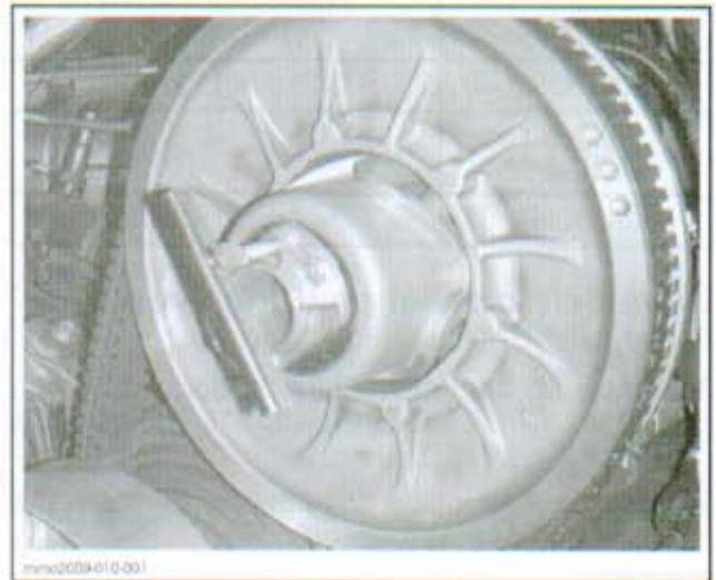
DRIVEN PULLEY OPENING TOOL (IN TOOL KIT)
