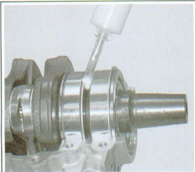
PTO SIDE BEARING FILLED WITH GREASE
