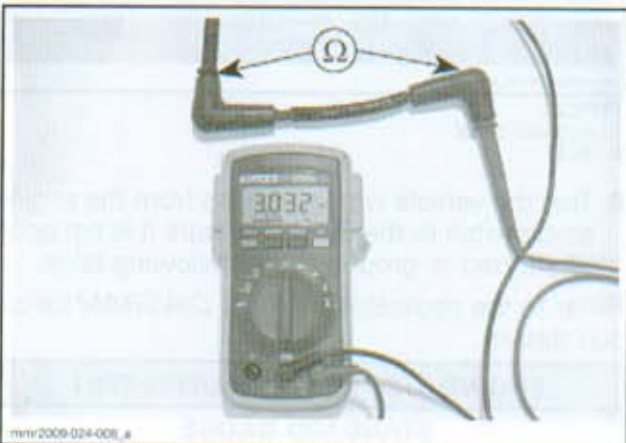
SPARK PLUG CABLE RESISTANCE TEST
