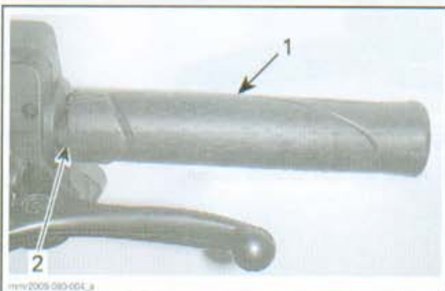
TYPICAL - LH SIDE 1. Grip with integrated heater element 2. Heater wire
