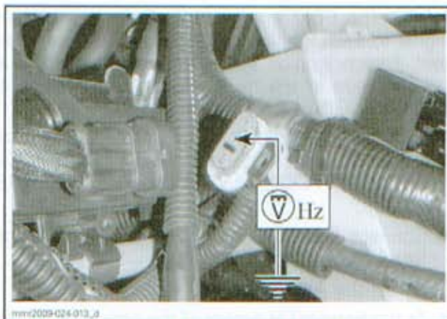
IGNITION SIGNAL TEST AT COIL CONNECTOR
