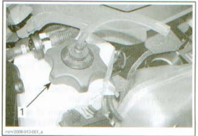
TYPICAL 1. Test cap on tank
