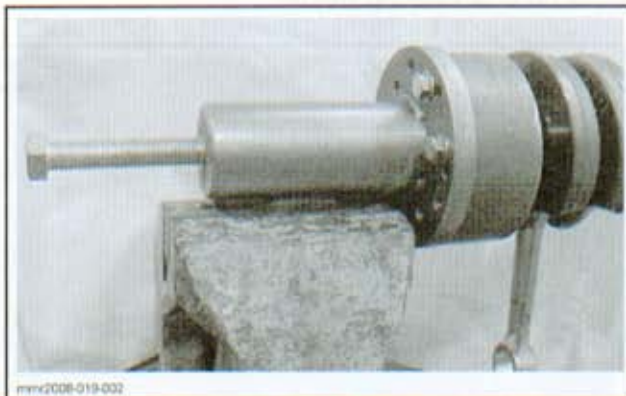
BEARING PULLER SECURED IN THE VISE
