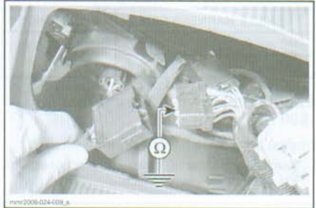
TYPICAL - VEHICLE HARNESS TO GROUND
