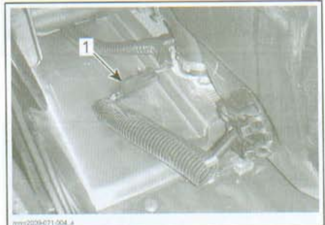
1. Fuel level sensor connector to disconnect
