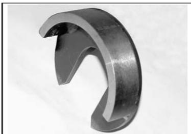
Distance gage for bearing on crankshaft
