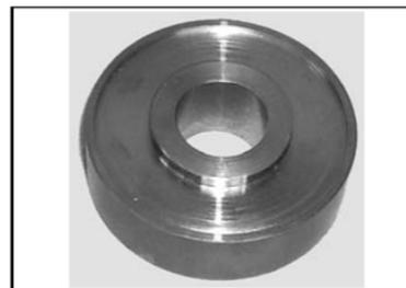
Engine support bearing installer
