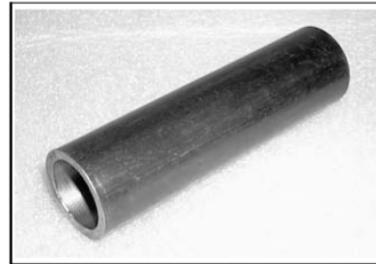
**Crankshaft MAG bearing installer**
