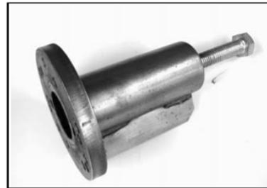
**Crank shaft bearing puller**
