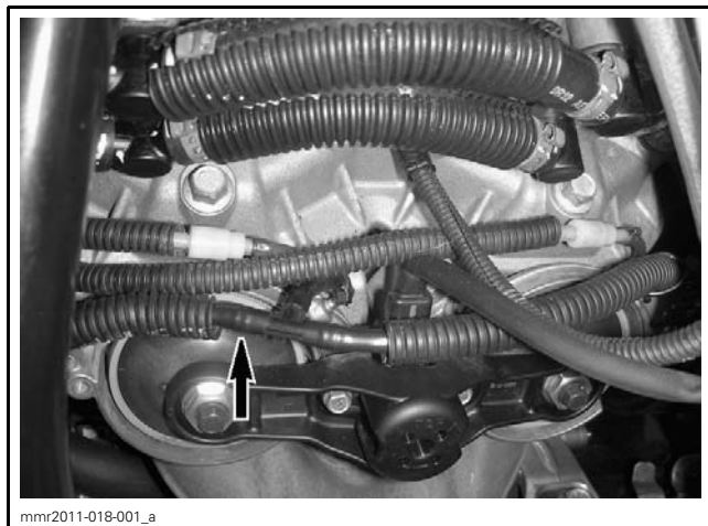
INLET HOSE AT T-FITTING
