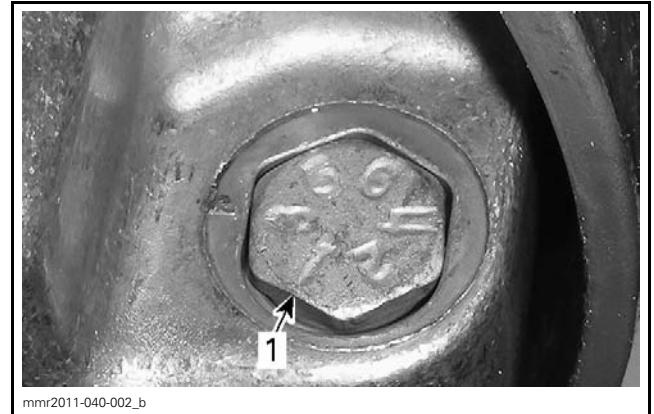
mmr2011-040-002_b CALIBRATION SCREW HEAD 1. Position 1
