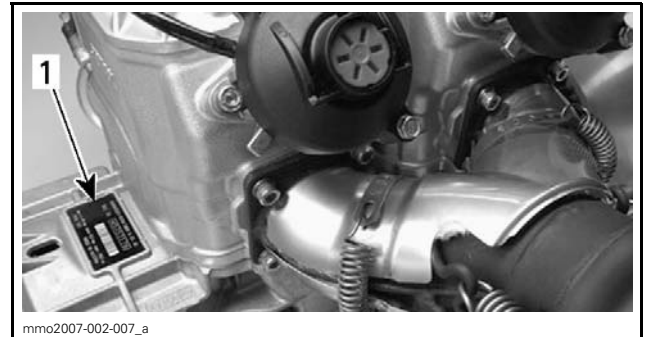
TYPICAL — 600 HO E-TEC 1. Engine serial number
