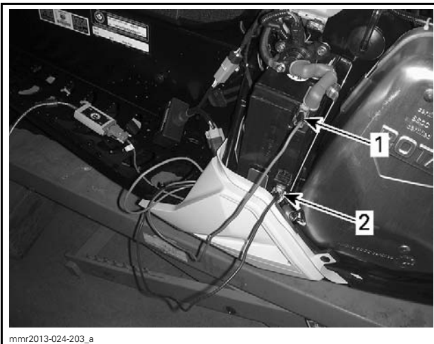
1. Red cable to battery "+" terminal 2. Black cable to battery "-" terminal
