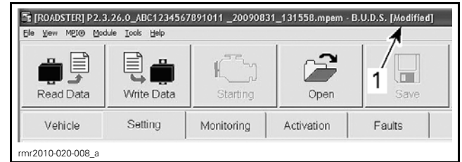
TYPICAL 1. Indicate setting or data modified; Write Data to save
