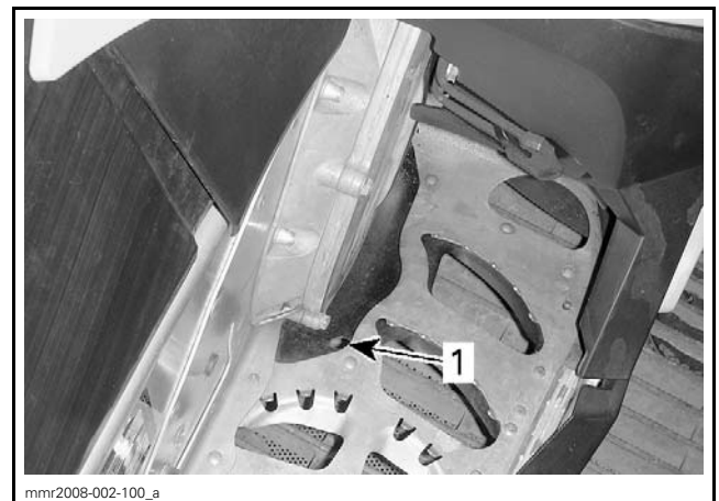
1. Reinforced holes in footrest
