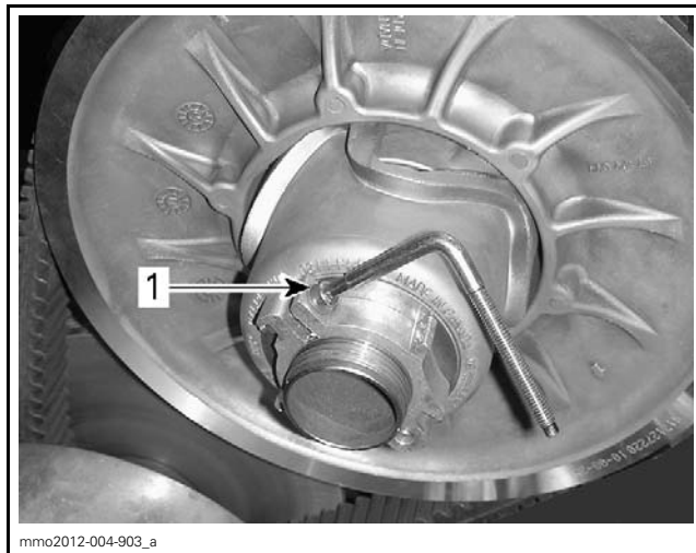
TYPICAL 1. Clamping screw
