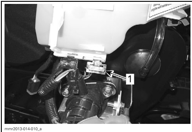
1. 25 A fuse location
