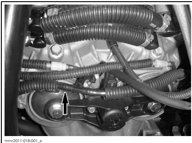
INLET HOSE AT T-FITTING
