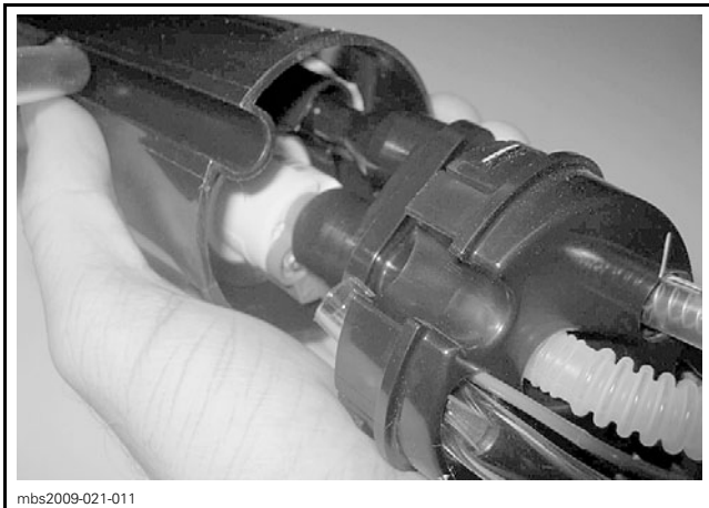
STEEL MESH FILTER, FUEL PUMP REMOTE PICK-UP
