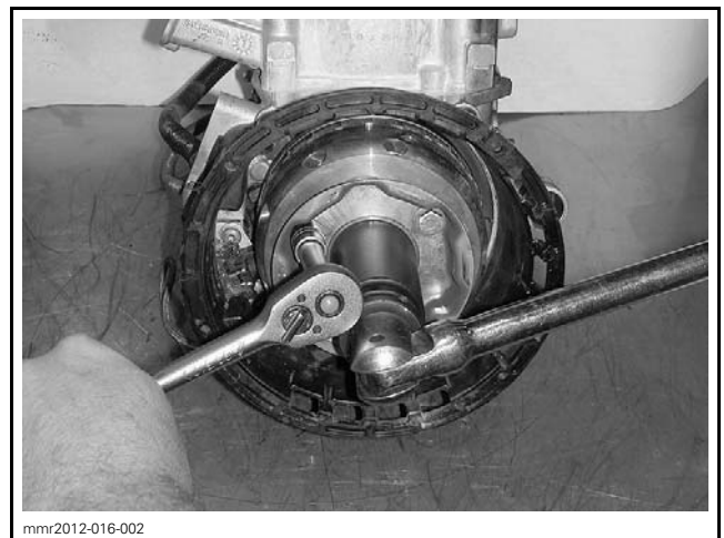
mmr2012-016-002 TYPICAL - STARTING PULLEY SCREWS REMOVAL
