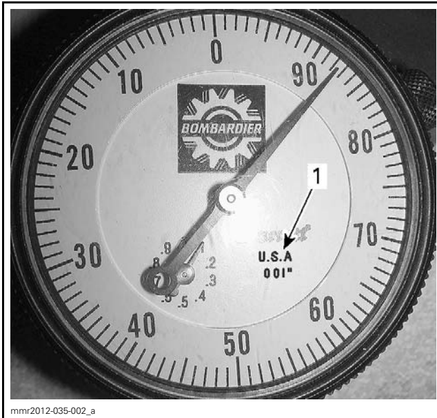
IMPERIAL GAUGE EXAMPLE 1. 001 inch means it is graduated each 1/1000 inch
