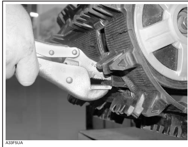
TYPICAL - PULL ON SLIDER SHOE TO REMOVE
