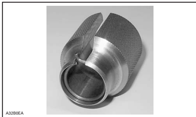
CIRCLIP READY TO BE INSTALLED ON PISTON
