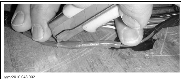
1. Broken wire stripped 2. Splice wire stripped
