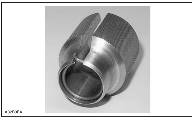
CIRCLIP READY TO BE INSTALLED ON PISTON
