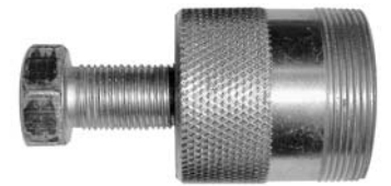
MAGNETO PULLER (P/N 529 035 547)
