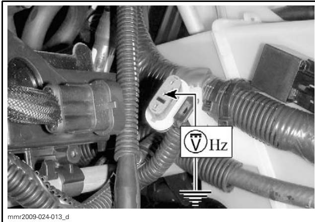
IGNITION SIGNAL TEST AT COIL CONNECTOR
