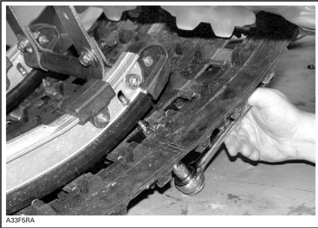
TYPICAL - REMOVE NUT AND SCREW OF EACH RUNNER
