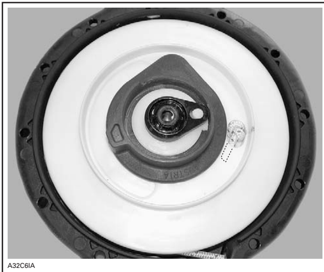
FREE PORTION INSERTED INTO SHEAVE
