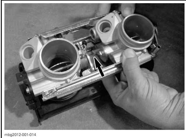
TYPICAL - PUSH TO OPEN THROTTLE PLATES
