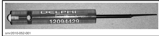
DELPHI TERMINAL EXTRACTOR (P/N 12094429)
