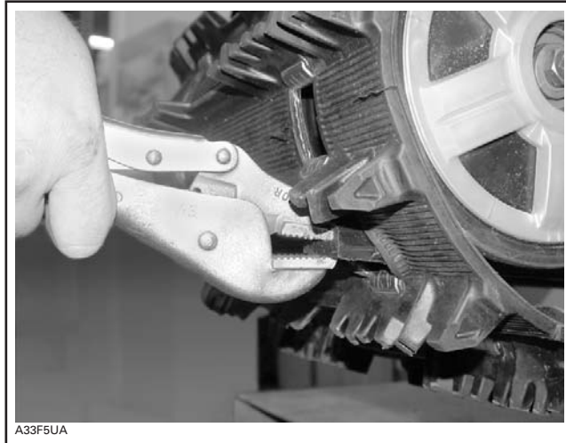
TYPICAL - PULL ON SLIDER SHOE TO REMOVE
