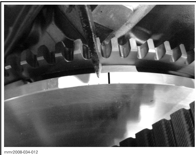
TYPICAL — TIMING ADVANCED BY ABOUT 2°
