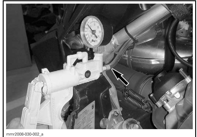
TYPICAL - VACUUM/PRESSURE PUMP ON VENT TUBE
