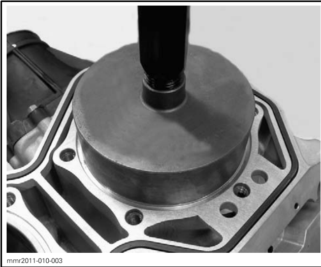
TYPICAL - TOOL PROPERLY CENTERED
