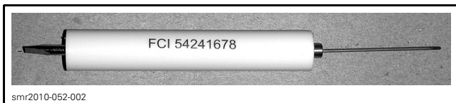
FCI TERMINAL EXTRACTOR TOOL (P/N 54241678)
