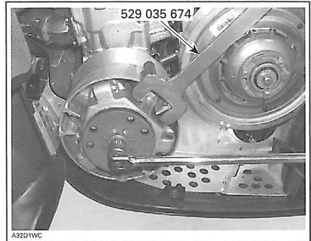
TYPICAL — INSERT THE TOOL IN SLIDING FLANGE CAVITIES
