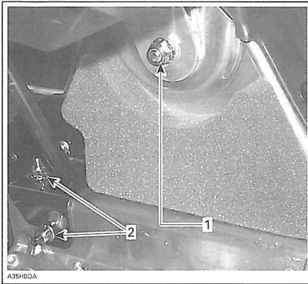
LH SIDE OF VEHICLE 1. Upper cross member nuts 2. Lower cross member nuts
