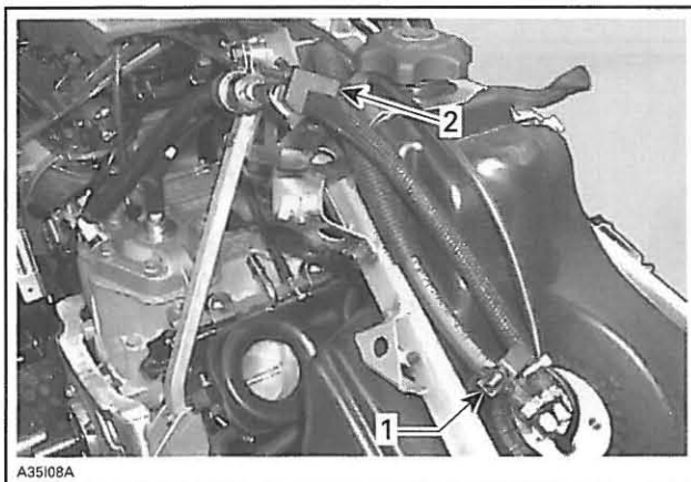
1. High pressure fuel pump INLET hose 2. High pressure fuel pump OUTLET hose
